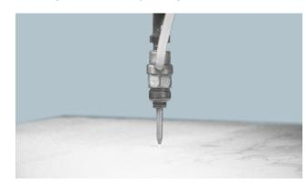
Laminated porcelain stoneware can be drilled with water jet cutting machines. With water jet machines, one can obtain holes with a smaller diameter compared to those possible with CNC machines. Operating speed must range from 2 to 3 m/min.
