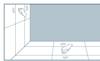
This test consists in an inspection of the tiling also by means of tapping in order to make sure that nothing has become detached or showing signs that detachment is starting to occur.
