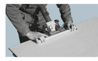
The use of the grinder together with particular trolleys allows the execution of flat chamfers with angles between 35° and 55° (with Jolly-angle type trolleys produced by Sigma) or round chamfers (with a Power-Raizor type trolley produced by Raimondi).
