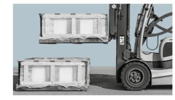
100x100 cm, 50x100 cm, etc.) must be handled one at a time. The forks must be supporting the entire depth of the pallet and be as far apart as possible. Forks must be at least 1.3 m long. During handling, take the appropriate care depending on the working conditions.
