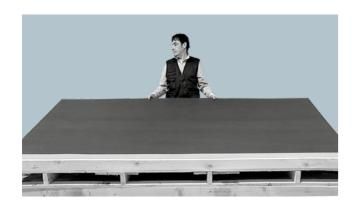
100x300 cm and 120x260 cm slabs of laminated porcelain stoneware can be lifted by one person. Lift the slab with open hands. Slowly raise the longer side so as to eliminate the suction effect, due to contact with the underlying slab, and ensure a good grip. When handling the use of gloves is recommended.
