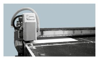
Laminated porcelain stoneware can be cut by scoring. This operation must be performed on a cutting bench and on the front face of the slab. In the case of 3plus, 5plus or 6plus laminated porcelain stoneware, if this operation cannot be performed automatically on a cutting bench, the fibreglass mesh must be cut by hand with a
