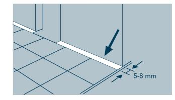
Around fixed elements of the supporting surface, such as walls, steps, columns, etc., it is mandatory to install 5-8 mm perimeter joints.
