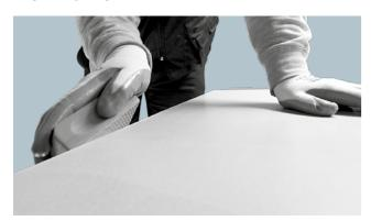
Edges can be finished by hand using abrasive diamond sponges or emery paper. By slightly sanding the side of the slab, one can obtain a slightly rounded-off edge and with repeated sanding one can obtain a bevelled effect.
