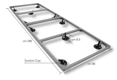
To safely handle and install 100x300 cm and 120x260 cm laminated porcelain stoneware slabs, a special frame is available upon request. It is made of aluminium and features suction cups. It is ideal for installing on scaffolding at a height of over 2 metres.
