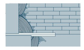
If there are joints between surfaces of different types (e.g. reinforced concrete and bricks), it is mandatory to install an expansion joint.
