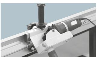
With the tile cutter rulers one can use hand-held angle grinders, fitted into a special frame (such as Power-Raizor by Raimondi) that guides it during the cut.
