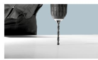
As far as manual drilling is concerned, use tungsten bits with a diameter up to 10 mm, fitted to electric drills or battery-operated screwdrivers.
