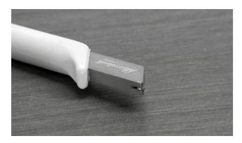
It is possible to obtain excellent results in terms of clean shapes and cuts by scoring all versions of laminated porcelain stoneware with products like Silberschnitt 2000 special glass cutters made by Bohle Italia or manual tile cutters made by Würth.
