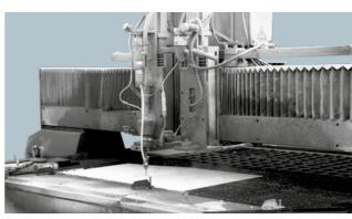
Laminated porcelain stoneware can be cut with water jet cutting machines. The feed rate of this operation should be between 2 and 3 m/min.
