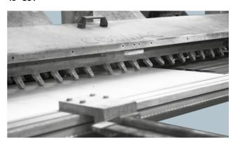
To obtain 45° cuts, use 45° diamond discs. In this way, it is possible to join two slabs of laminated porcelain stoneware to create a corner. The corner achieved must then be bevelled. Different discs are available for obtaining a variety of edge finishes. Operating speed must be tested beforehand.
