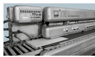
To shape the edge, first of all use abrasive diamond wheels which are suitable for obtaining the required shape and size. A polishing wheel must then be used for polishing. By using different grinding wheels it is possible to obtain numerous types of edge finish. Operating speed must be tested beforehand.
